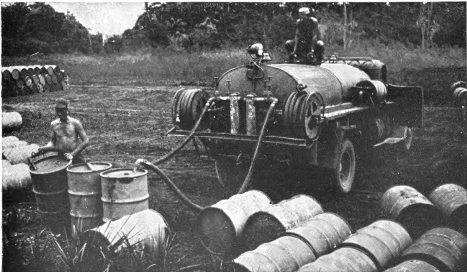
Figure 139. Pumping gasoline from 55-gallon drums to tank truck.
